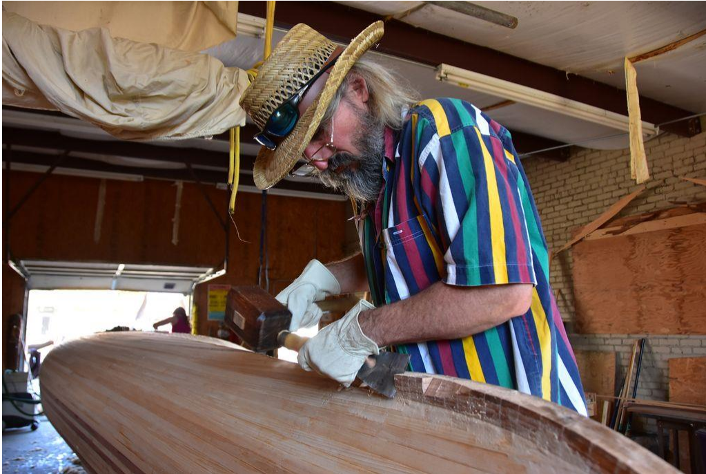
Driftwood Johnnie Shaping the Stern with a 3" Flat Carving Chisel & Wood Mallet
